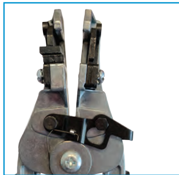
Short-stop latch protects wire strands by limiting the stripping stroke to 4 mm (5/32") and retains the slug until the wire is ready for termination
