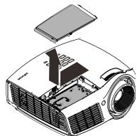
4) Remove the three screws from the lamp module.
