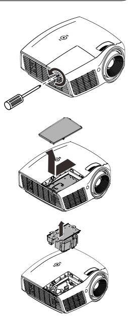
6) Reverse steps 1 to 5 to install the new lamp module. While installing, align the lamp module with the connector and ensure it is level to avoid damage.
