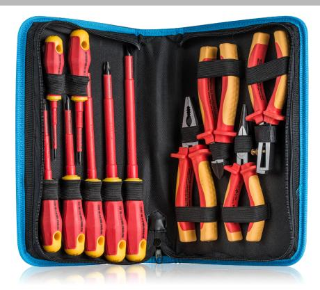
These tools are made of heat treated chrome vanadium steel for maximum strength and durability. The tools meet or exceed IEC 60900, ASTM F1505-01, and VDE standards for high voltage protection and are tested to 10,000 VAC and rated to 1,000 VAC live use.
