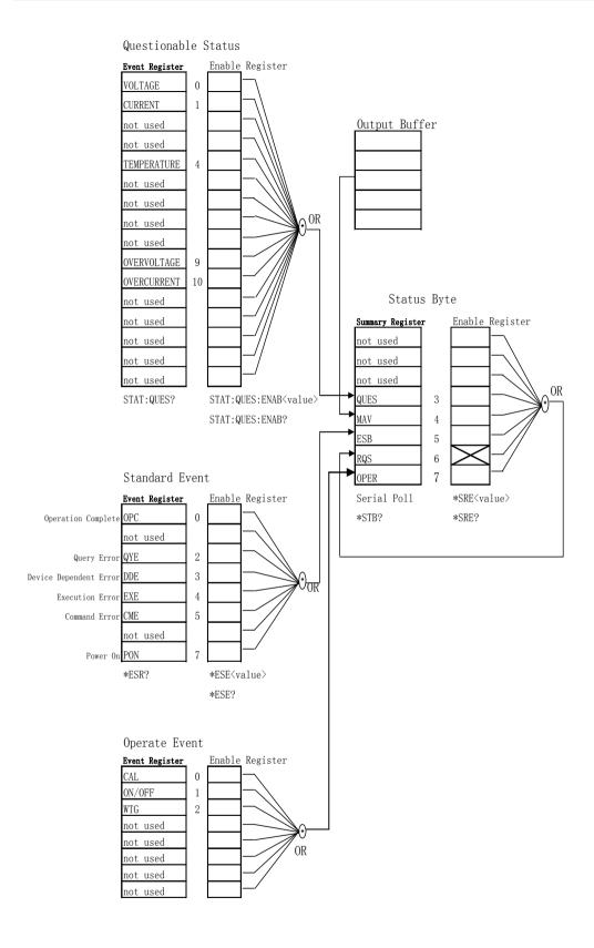
Event register is read only register, used to store the implementation status of the power, the data used in the event register latches in the form, once the data is stored, subsequent data will be completely ignored. Even can't changed by re-setting order (\* RST) or equipment restart.
