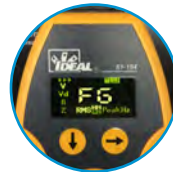
Detects and Displays false or "bootleg" ground
