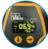
Displays Voltage Drop at 12, 15 & 20 Amps
