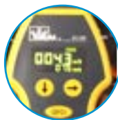
Trips GFCI at 6mA or 30mA
