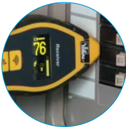
Finding Breakers or Fuses
