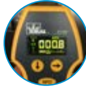
Displays neutral to ground voltage
