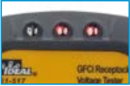
Red Lights Indicate Incorrect Wiring
