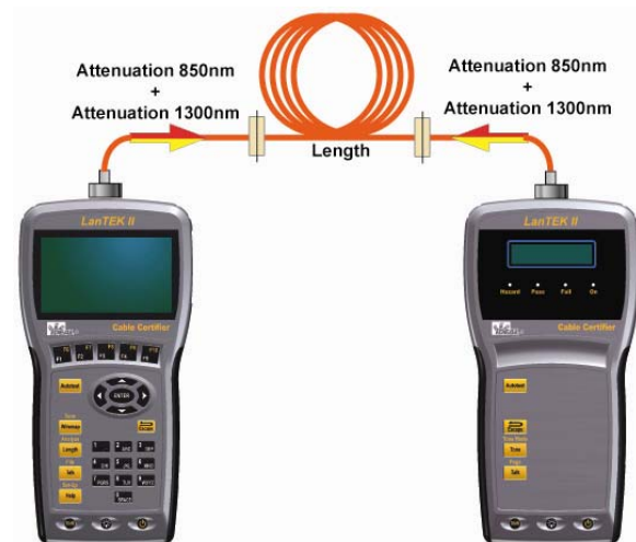
Figure 5: FiberTEK® FDX bi-directional testing without mandrels
