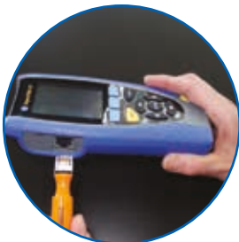
Replaceable RJ45 contacts
