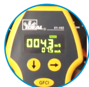
Trips GFCI at 6mA or 30mA
