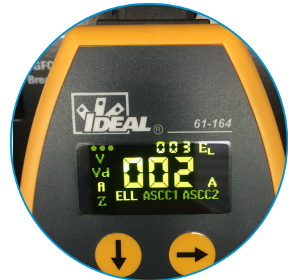
Estimated Load on Line in Amps
