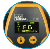
Detects and Displays false or "bootleg" ground
