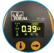
Displays Impedance of hot, neutral & ground
