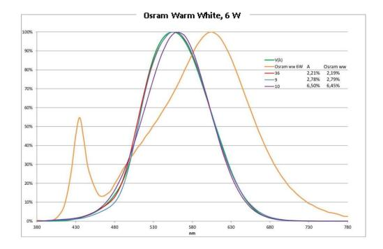
As we can see, error does not change for this LED with matching to the sensitivity of the human eye. For all three filterings, error with  $V(\lambda)$  matching is practically identical to error for light type A.
