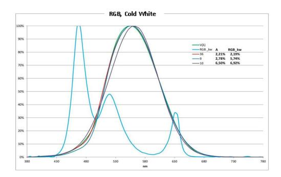
For these two white LEDs, by means of which white light is generated by variably controlling one red, one green and one blue LED, filtering error is greater relative to light type A, although it's not yet significant.
