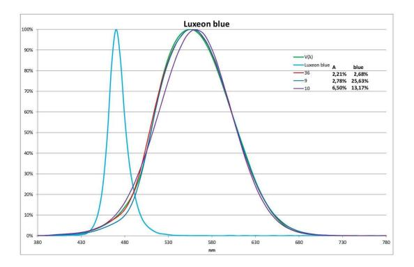
In the case of the blue LED with filter no. 9, a considerable difference relative to error with light type A becomes apparent.
