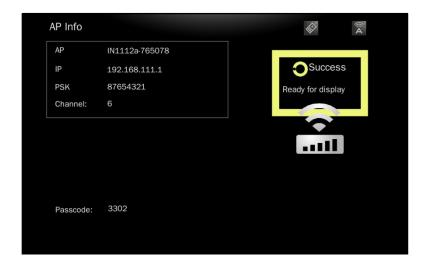
4. From the PC, open the WiFi SSID list and select the access point indicated in the Welcome page. Enter the displayed PSK if encryption is enabled.
