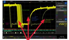
Infrequent glitches and signal jitter captured after 1 second on the 3000T X-Series with standard 1M wfms/s update rate.
