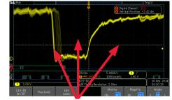
MD03000 after 30 seconds with infinite persistence on. It shows limited signal jitter and never sees the glitches due to its compromised update rate.
