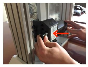
**Step 11** Route the power cable (C) coming from the actuator motor out the back of the unit through the notch in the back cover and attach the power cord extension.
