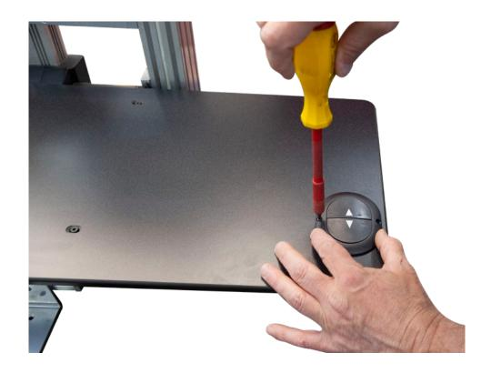
**Step 10** Plug the connector from the switch located on the top work surface to the port on the left side of the actuator motor as shown below.
