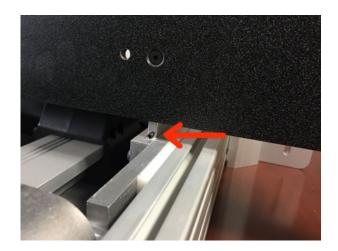
**Step 6** Hand tighten the thumb screws fully to secure the work surface into place.
