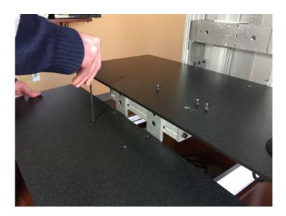
**Step 13** Screw the lower work surface on to the right angle brackets with the flat head screws (B) and the supplied 4mm allen key.
