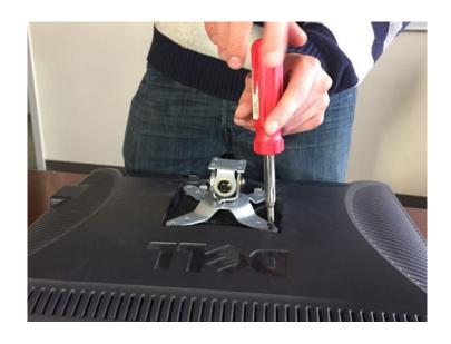
Step 16 One attached, slide monitor pivot into the pivot pocket located on each arm.
