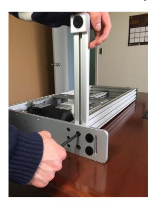
**Step 4** Loosen the screws in the middle of the work surface support brackets as shown here. These screws may be loosened with the included #5 allen key or by hand based on preference.
