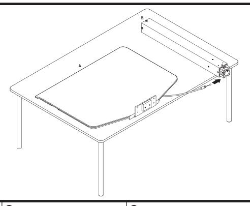
Confirm cable is properly seated into position.
