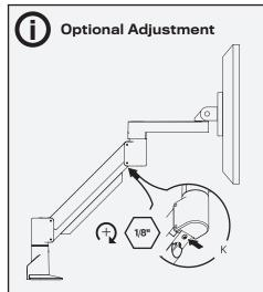
**In some instances,** an additional counterbalance adjustment may be needed to allow the arm's instant height adjustment function to work properly.
