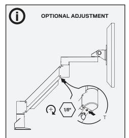
In some instances, an additional counterbalance adjustment may be needed to allow the arm's instant height adjustment function to work properly.
