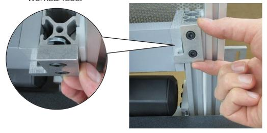
**Step 10:** Tighten bolts with 5mm hex key.
