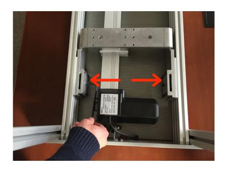
**Step 5:** Slide the upper worksurface (F) into the support brackets as shown:
