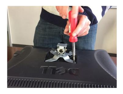
**Step 19:** One attached, slide monitor pivot into the pivot pocket located on each arm.
