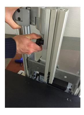
**Step 18:** Attach monitor to pivot (L) using provided Phillips head screws (M).
