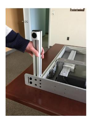
**Step 3:** Re-tighten the screws at the base of the unit to secure the legs to the base.
