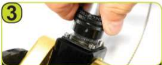
3 Connect the crawler to the mainline cable receptacle.
