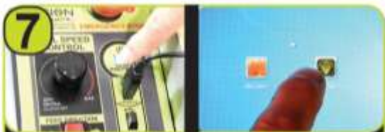
7 Press the power button on the face of the system. Select User option on boot-up screen (admin for service only).
