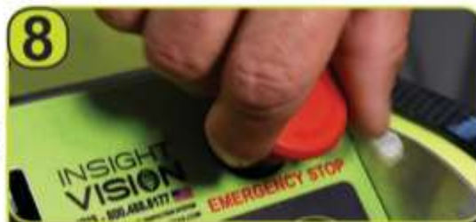
8 Turn E-Stop Clockwise to turn on crawler.
