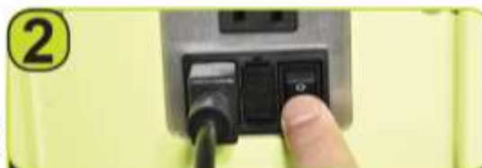
2 Plug in the power cable on the back of the system and switch the power toggle to the ON position.
