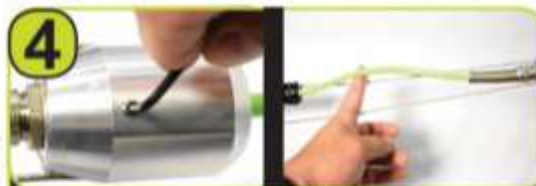
4 Tighten strain relief clamp using the provided allen wrench. Assure there is slack in the cable between strain relief and connector.
