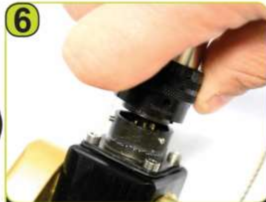
6 Screw counter clockwise to disconnect crawler from cable.
