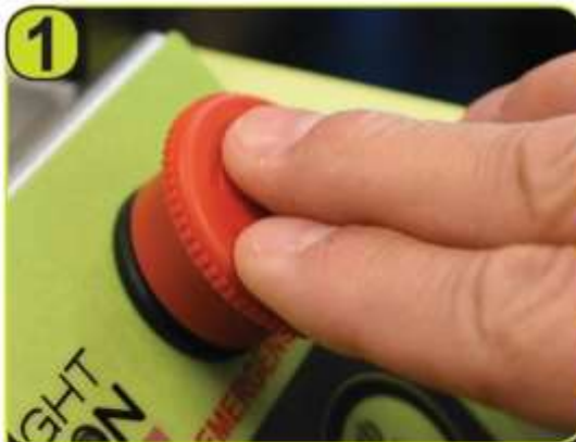
1 Push in the emergency stop to shut off power to the crawler.
