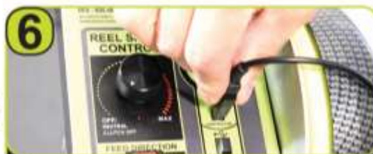
6 Plug in the crawler controller into the specified USB controller port.
