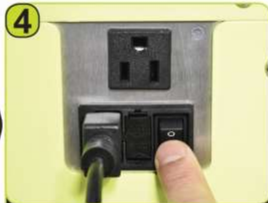
4 Press Power OFF on the back of the reel and unplug the power.
