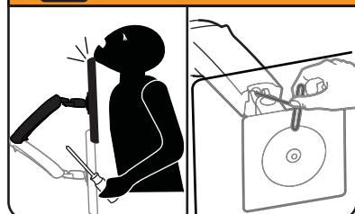
WARNING! Stored Energy Hazard: The arm mechanism is under tension and will move up rapidly, on its own, as soon as attached equipment is removed. For this reason, DO NOT remove equipment unless the arm has been moved to the highest position! Failure to follow this instruction may result in serious personal injury and/or equipment damage!
