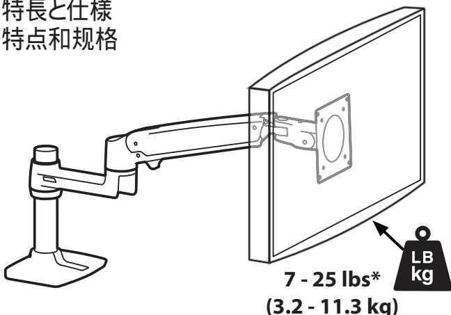
\* The lower most range of motion for vertical lift is decreased up to 4.5" (114 mm) when arm is adjusted to hold over 20lbs (9 kgs).
