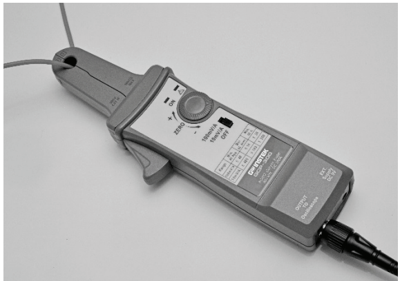
Figure 2. Connecting the GCP-300 current probe.
