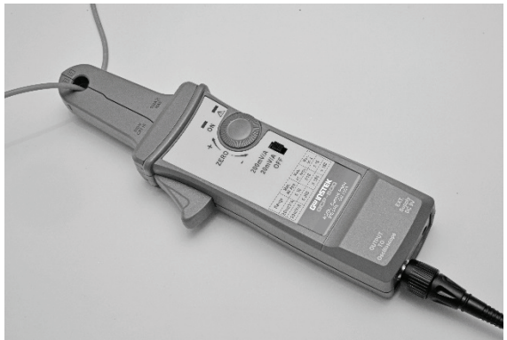
Figure 2. Connecting the GCP-300 current probe.
