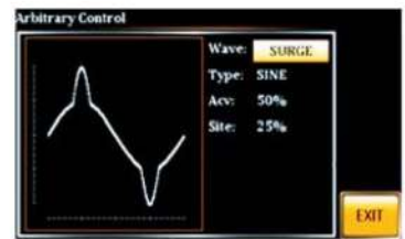
Surge Waveform Simulate Grid Power Supply's Peak Over-voltage
