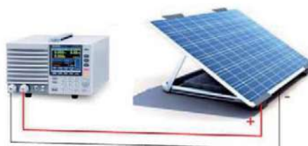
Connections Between PEL-3041 and Solar Panel
