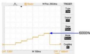
PEL-5006G-150-600 Turbo mode OFF OPP Pstep 50W, Pstop 6000.0W real test waveform
