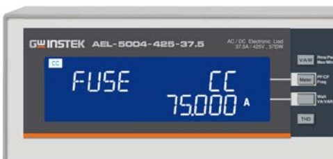
Turbo : OFF, Fuse mode Test result screen
