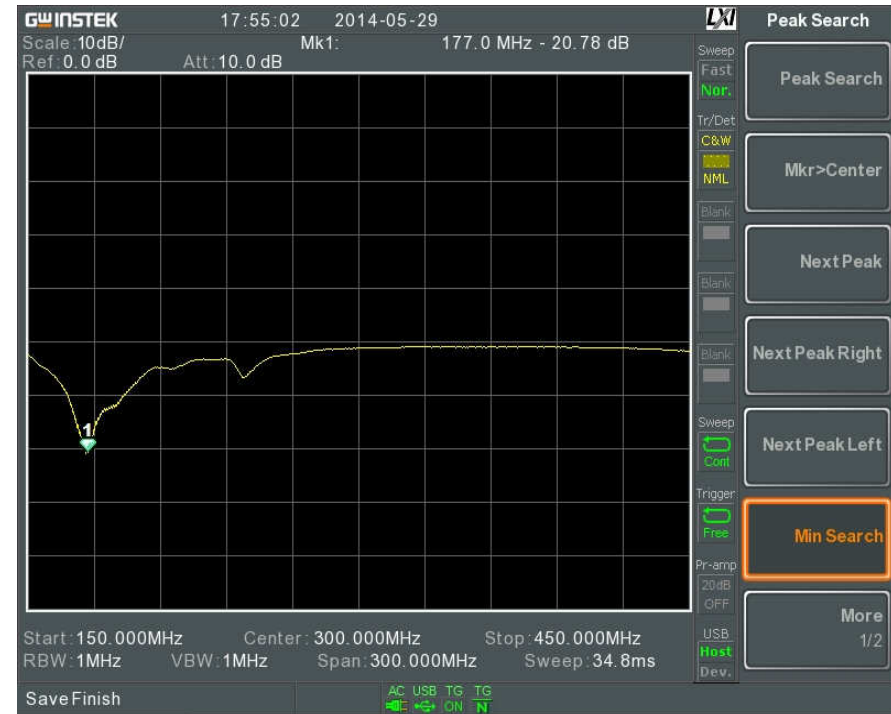
Antenna Return Loss Testing
