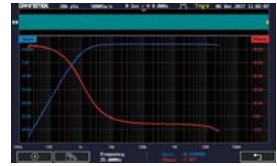
FRA of RC high-pass filter
