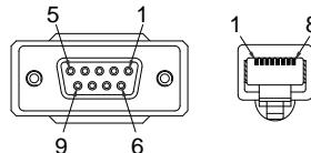
RS485 cable with DB9 & RJ-45 shielded connectors from GTL-260 connection kit
