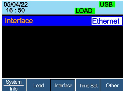
3. If the interface is not set to Ethernet, use the selector knob to change the interface to Ethernet.
