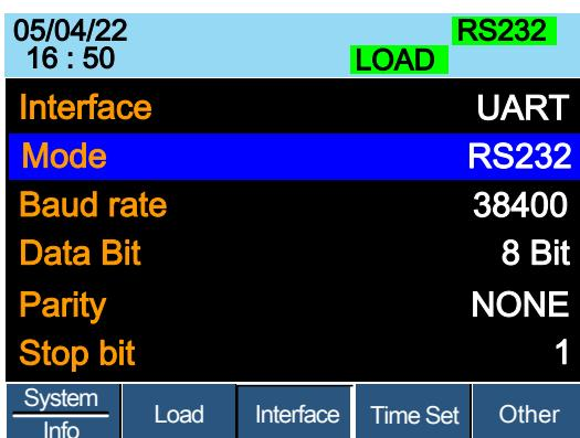
4. Edit the Baud rate, Stop bit and parity.
