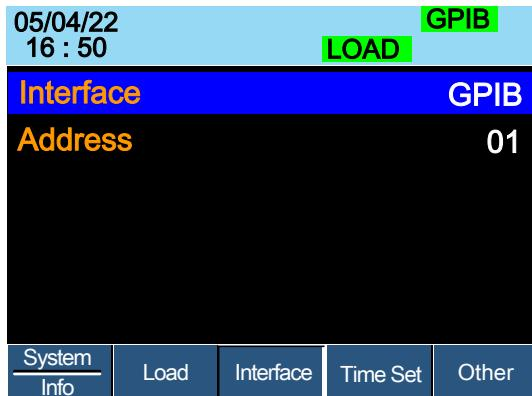
3. If the interface is not set to GPIB, use the selector knob to change the interface to GPIB.
