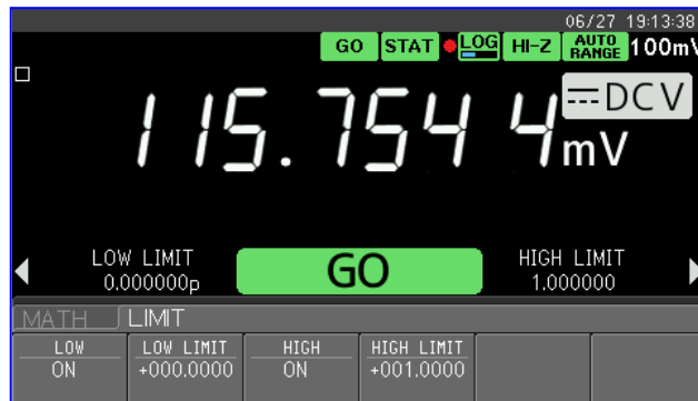
Figure 2.18 Example of LIMIT calculation result display (VOAC7602)
