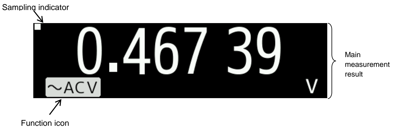
Figure 2.11(f) Example of NUMERIC display (FONT :NORMAL, VOAC7502)
