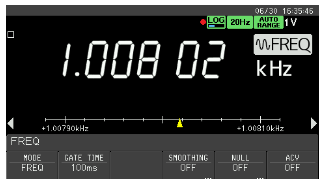
Figure 3.9(b) Frequency measurement (FREQ) screen
