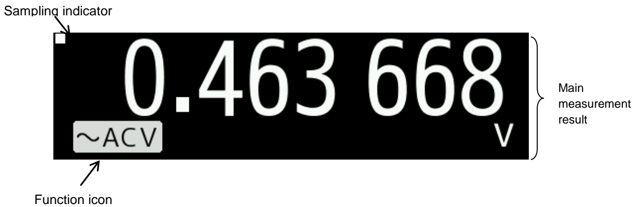
Figure 2.11(e) Example of NUMERIC display (FONT :NORMAL, VOAC7602)
