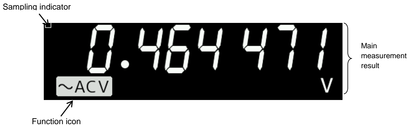
Figure 2.11(d) Example of NUMERIC display (FONT :7SEG, VOAC7602)
