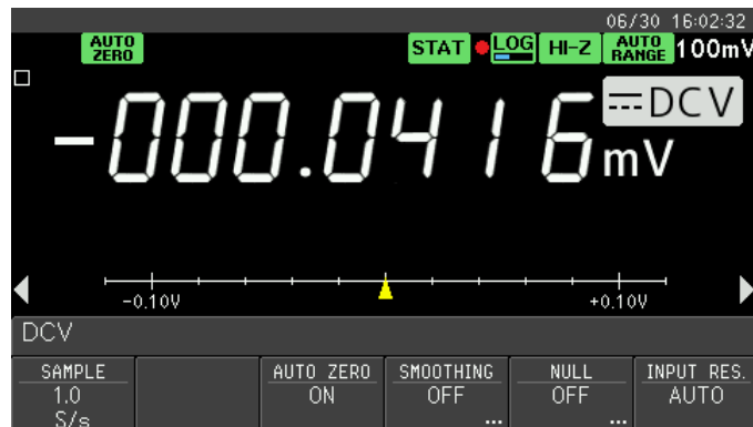
Figure 3.4 Screen display at startup (VOAC7602)
