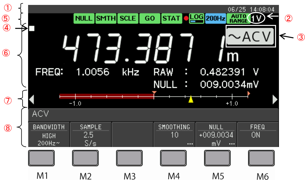
Figure 2.8(a) Example1 of VOAC7602 (PRIMARY: NUMERIC, SECONDARY: ANALOG METER)
