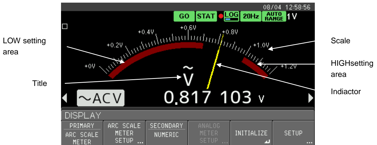
Figure 2.15 Display example of ARC SCALE METER (NUMERIC)
