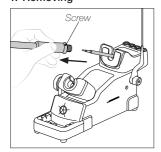
Loosen the handle screw. Place the Soldering Iron with the cartridge in the extractor and pull the handle to remove ...
