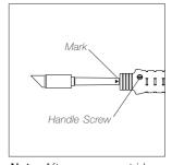
**Note:** After proper cartridge insertion as far as the mark ►I, tighten the handle screw.
