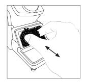
Replace the brass wool with a new one when it is worn out.
