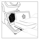
Remove the wiper by pulling it out.
