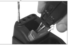
Place the cartridges in the extractor and pull the tweezers to remove them.
