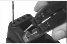
Use the grooves to insert the cartridges as far as they stop.
