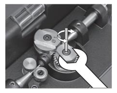
**2.** Replace the guide wheel and the blade for the new ones.
