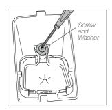
Loosen the screw and remove the screw, the washer.
