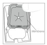
Finally the membrane. Replace the membrane for a new one.
