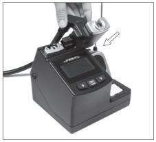
2 Insert the fume inlet duct for compact stations between the knob and the tool holder.
