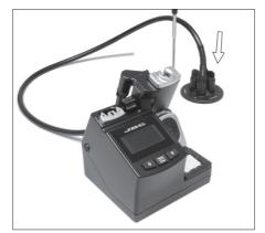
3 Connect the fume inlet duct for compact stations to the accessory for stand aspiration (Ref. FAE030/FAE040).
