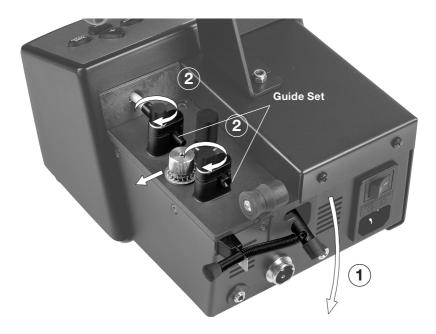
**3.** Insert the guide set in the tool. You must leave a gap of 8-10 mm between cartridge tip and the end of the guide tube.
