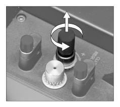
**3.** Pull out the standard driver gear supplied with the station.
