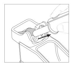
Place the heating element with the assembled nozzle in the nozzle changer and pull the tool to remove the nozzle.
