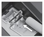
Push the cartridge into the handle to the mark\*.
