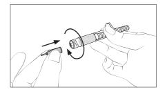
Thread the tip\* onto the syringe barrel.
