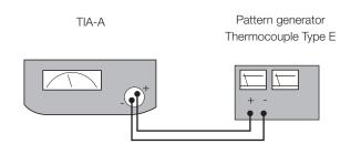
3. Choose the temperature on the generator and take a reading on the thermometer.
