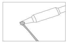
The soldering tip must be properly tinned before taking a measurement.
