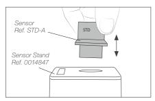
To replace the STD sensor, pull it vertically out of the sensor stand and replace it with a new one.
