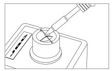
Place the soldering tip in the centre of the sensor as when soldering. Wait until the temperature measurement stabilizes.
