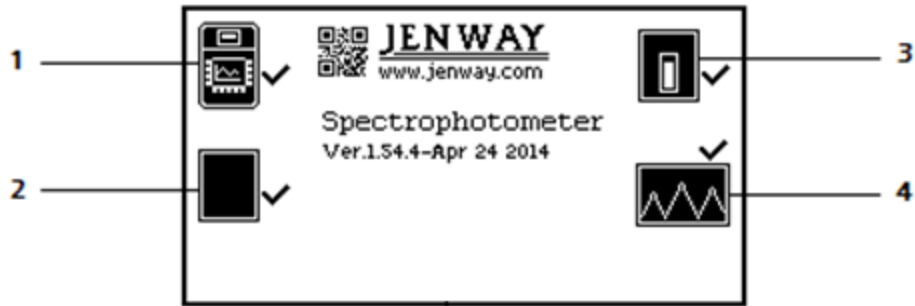
Fig 2.2.2 – All Power On Tests Complete
