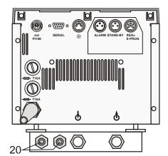
For applications near the ambient temperature, the cooling coil (20) must be connected to the water mains.
