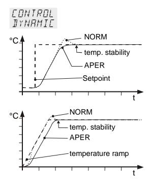
This parameter affects the temperature sequence only in case of internal control.
