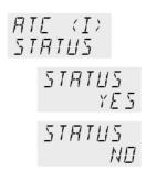
In the second submenu the ATC function for the temperature sensor selected above is activated >YES< or deactivated >NO<.
