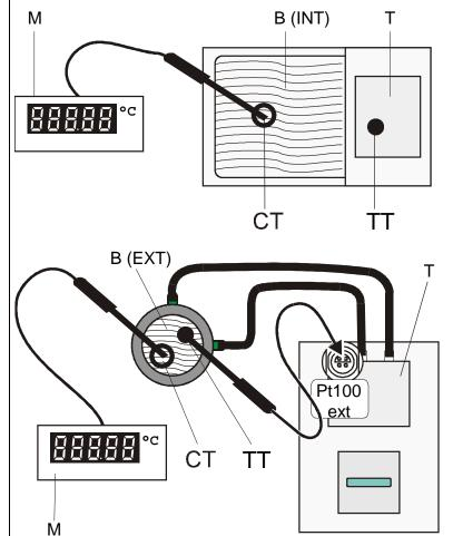
M = Temperature measuring instrument with temperature sensor
