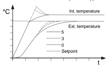
As soon as a co-speed factor is set, it is considered for calculating the control parameters. As shown in the diagram, tuning times become shorter the higher the co-speed factor is, but overshooting can happen in the internal system.
