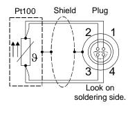
The shield of the connecting cable is electrically connected to the plug housing and the sensor tube.
