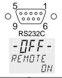
Check the interface parameters for both interfaces (on circulator and PC) and make sure they match. (Serial interface refer to page 48)
