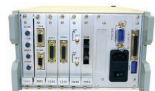
Model 1560 has 6 slots for modules
