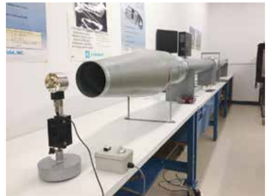
Wind Tunnel setup at Kanomax calibration lab
