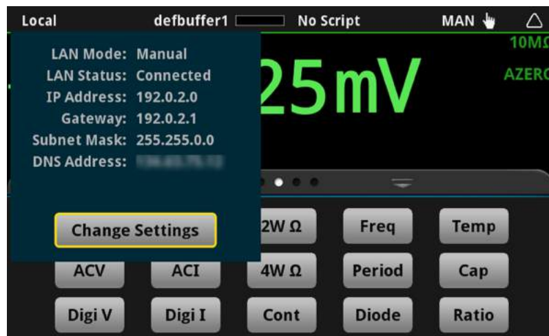
Figure 31: Communications indicator expanded
