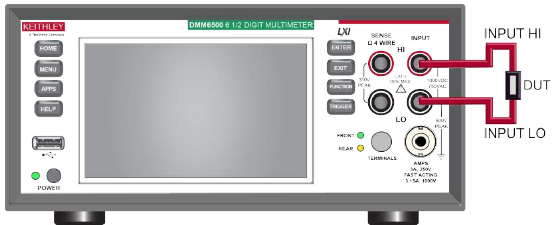
Figure 72: Two-wire DUT connections to the front panel
