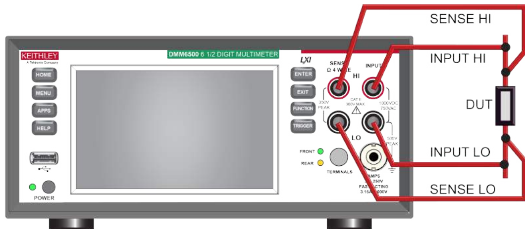
Figure 74: DMM6500 front-panel 4-wire remote sense connections
