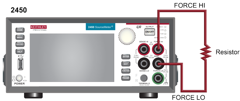
Figure 19: Model 2450 2-wire front-panel connections
