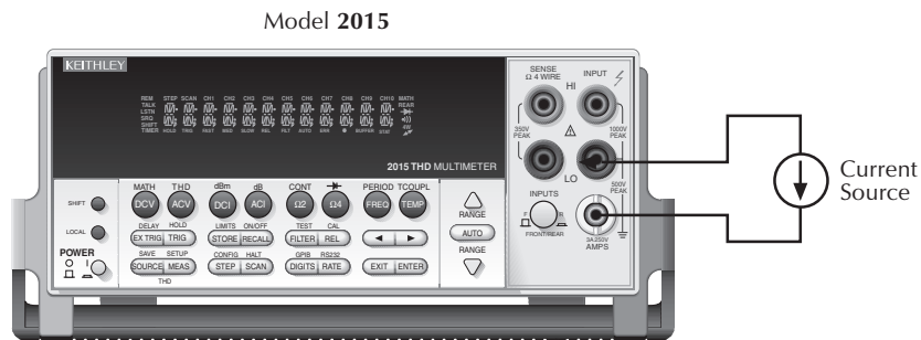
Figure 2-5 DC and AC current measurements
