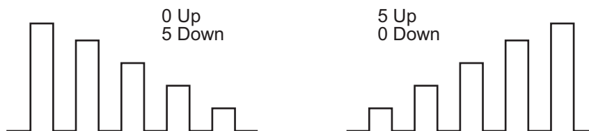
Figure 3-7 Sample one-shot only pulses for step method
