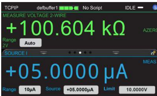
Figure 67: Resistance measurement SIMV SCPI example
