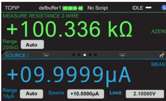
Figure 70: Resistance measurement with automatic settings
