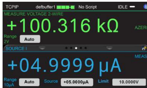
Figure 68: Resistance measurement SIMV and read ohms
