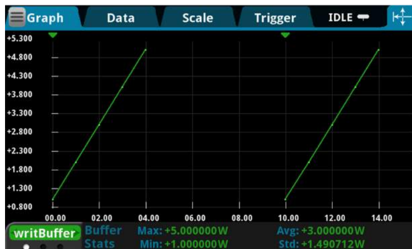
Figure 114: Graph with data from a writable buffer with start group markers
