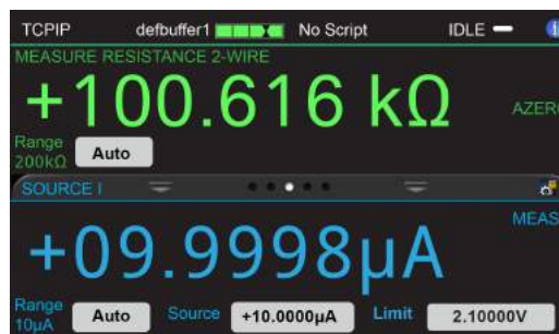
Figure 69: Resistance measurement using resistance function
