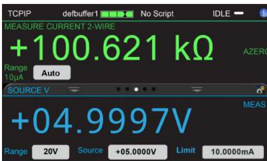
Figure 65: Resistance measurement using SVMI and reading ohms
