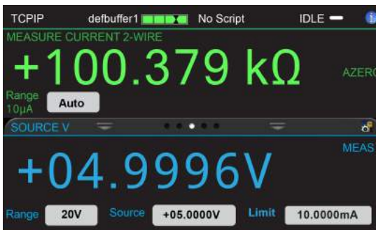
Figure 66: Resistance measurement SVMI and reading ohms
