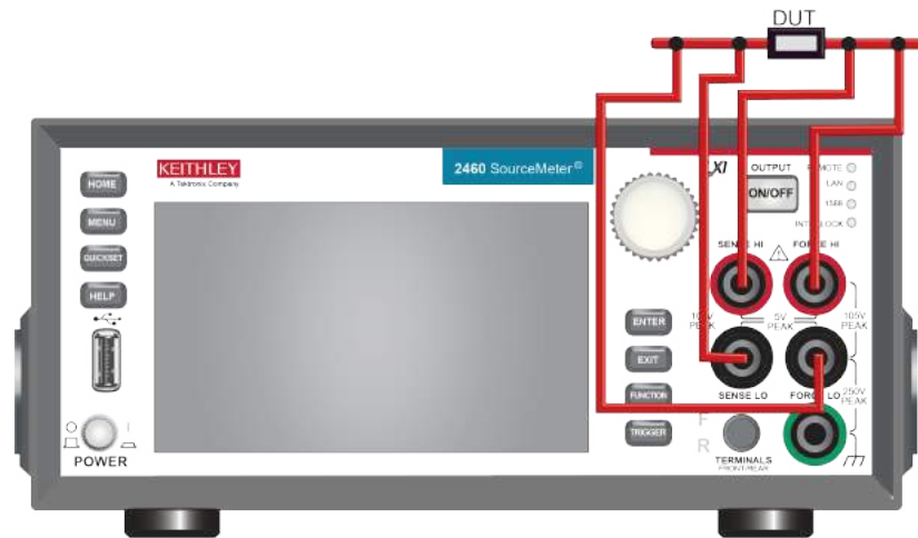
Figure 61: 2460 4-wire sense front-panel connection
