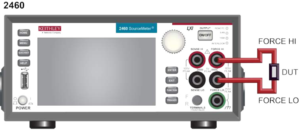
Figure 59: 2460 2-wire rear-panel connections
